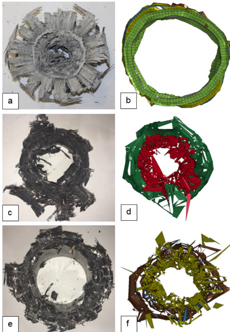
Figure 7-12 Plane view of GFRP and CFRP a) GFRP quasi-static Stitched experiment b) GFRP quasi-static stitched FEA c) CFRP quasi-static non-stitched experiment d) CFRP quasi-static non-stitched FEA e) CFRP quasi-static stitched experiment f) CFRP quasi-static stitched FEA
