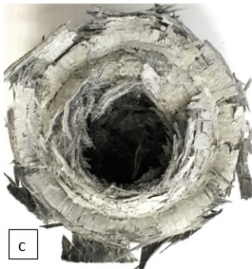
Figure 4-9 plane view of crushed multi-stitched composite sections, a) 10-20 mm, b) 10-30 mm, c) 20-30 mm.
