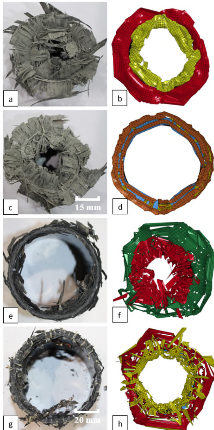
Figure 7-15 Plane view of GFRP and CFRP under impact loading a) GFRP non-stitched FEA b) GFRP non-stitched experimental c) GFRP stitched FEA d) GFRP stitched experimental e) CFRP non-stitched FEA f) CFRP non-stitched experimental g) CFRP stitched FEA h) CFRP stitched experimental
