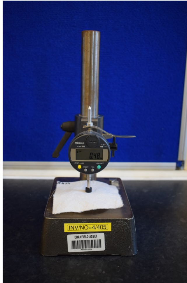
Figure C-2 a fabric sample on the thickness gauge
