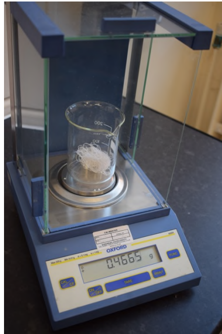
Figure C-3 measuring the linear density of ten yarns
