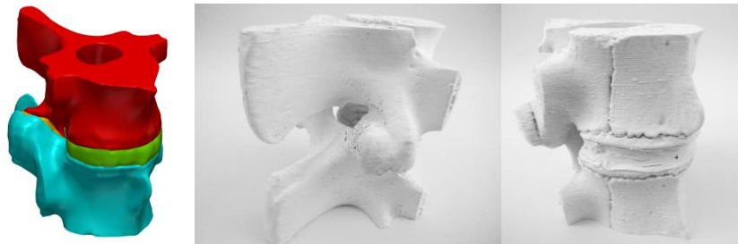
Figure 6-3 Artificial motion segment surface model and finished sample.
