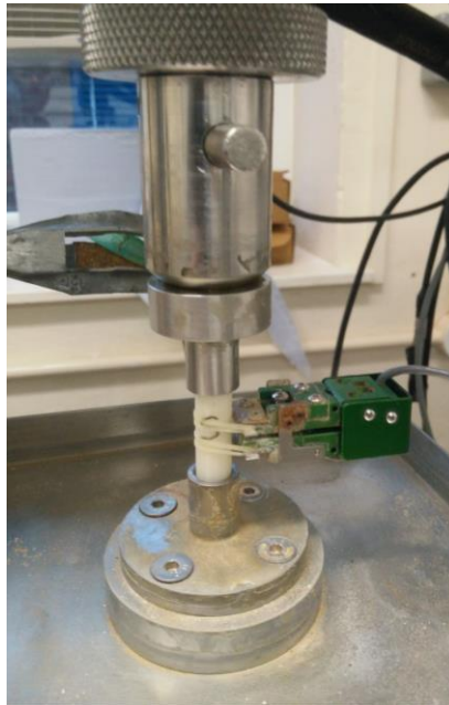
Figure 6-5 Mechanical testing setup with the top spherical joint endcap platen and the bottom fixed endcap platen.
