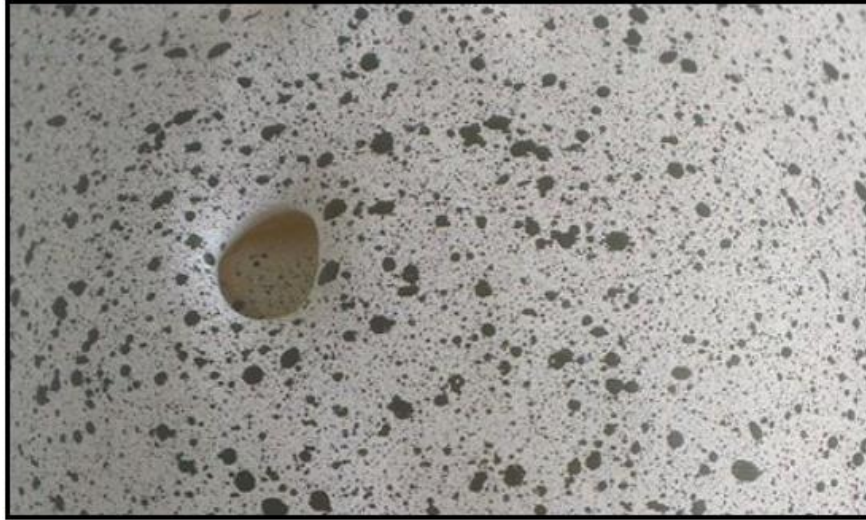
Figure 2-2 Typical speckle pattern, exemplified using a model with an excision to show the brain simulant within.
