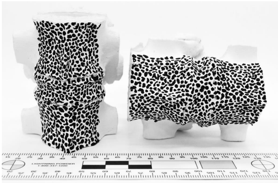
Figure 4-3 Speckle pattern applied to AMS 4 and AMS 4ii.
