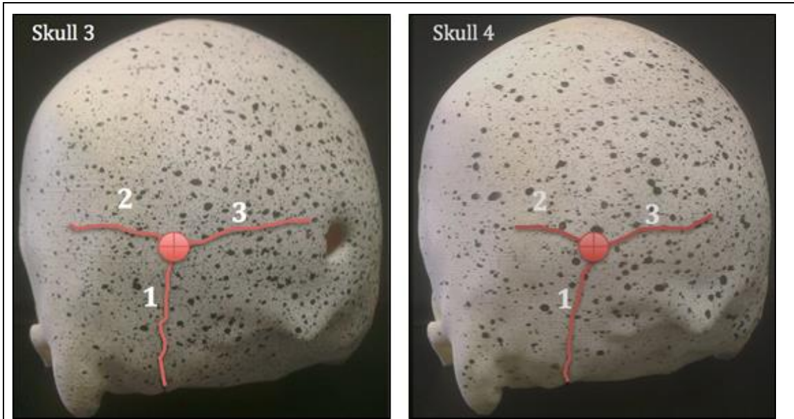
Figure 2-7 The initiation, propagation and magnitude of cracks under T2 test conditions in skull models with (left) and without (right) an excision.
