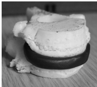
Figure 4-2 Moulding of the IVD analogue using PTFlex 70.
