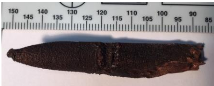
Figure 7-15. Recovered laser sintered slug.
