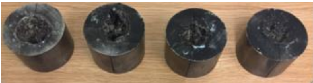
Figure 5-6. Surface entry hole produced by PLA jet in steel.
