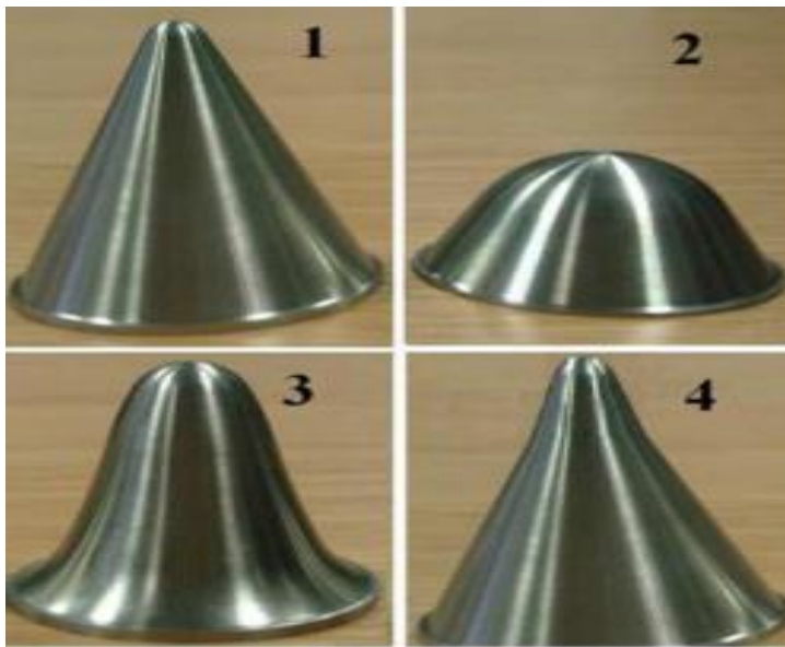
Figure 2-10. Picture showing different liner shapes. 1.conical 2. hemispherical 3. bell 4. trumpet or bi-conical [11].
