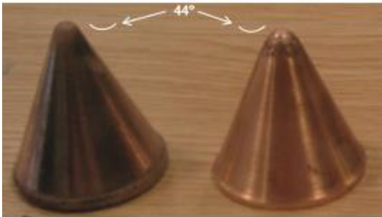
Figure 2-8. Pictures of the liners fabricated alloy; copper–tungsten liner powder (left) and the baseline copper (right) [36] .
