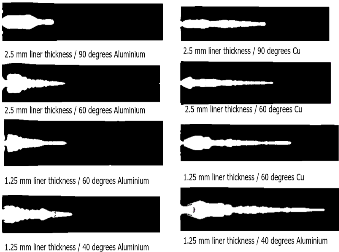
Figure 4-8. The penetration craters from Autodyn 2D numerical simulation.
