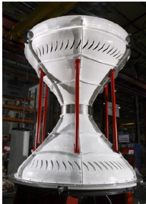
Figure 21: Part assembled VRT-2 prototype, (Natanzi et al. 2011).
