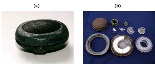
Fig. 8: Neutralised landmine. (a) External view. (b) Disassembled target [11]
