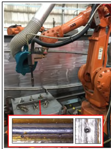
Figure 2. Manufacturing setup for the WAAM sample with the intentionally embedded tungsten carbide balls
