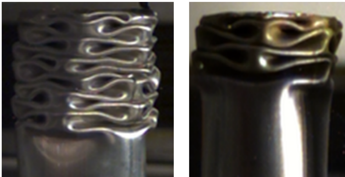
Figure 7 Deformed shapes of aluminium 6063 T6 and steel E235 tubes (Dimensions given in Table 1).
