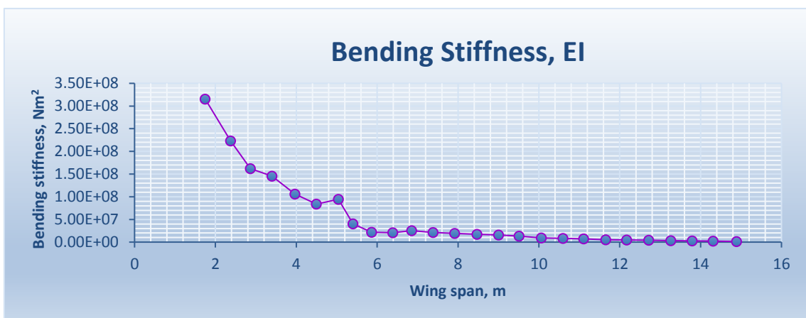
Figure 6.9 Bending stiffness distribution from NASTRAN
