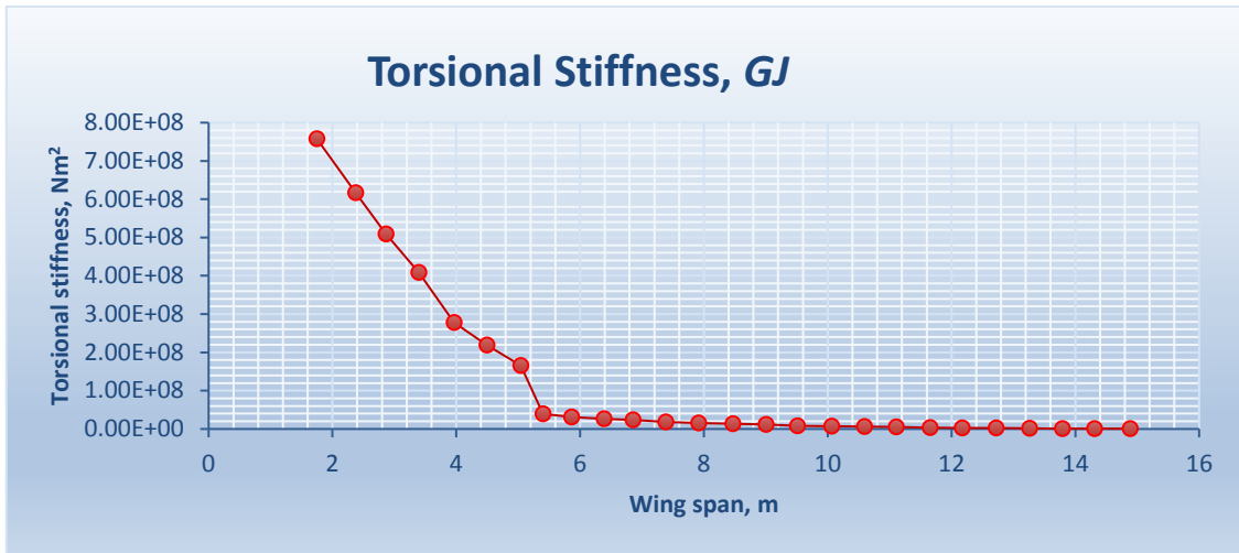
Figure 6.6 Torsional stiffness distribution from BOXMX Program
