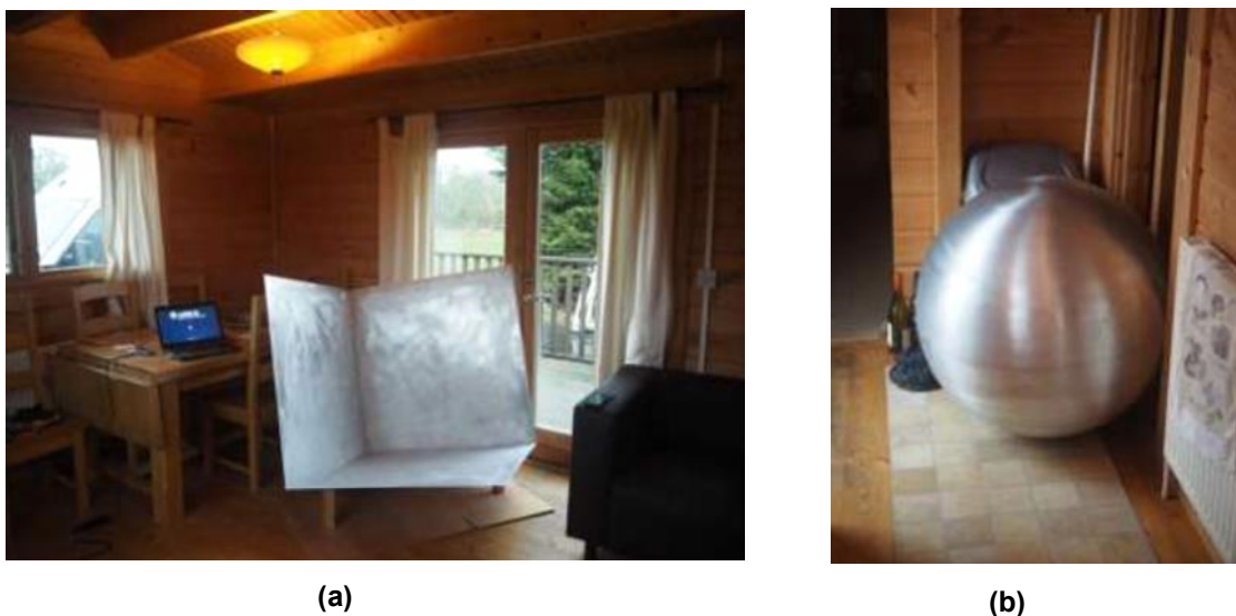
Fig 4. Calibration targets located within Arkle Lodge. (a) Square Trihedral: Azimuthal angle = 90^\circ , Elevation angle = 14.6^\circ , Height above ground = 1.5m, Latitude = 53.29196^\circ , Longitude = 0.27983^\circ . (b) Sphere: Height above ground = 0.6m, Latitude = 53.29191^\circ , Longitude = 0.027953^\circ .
