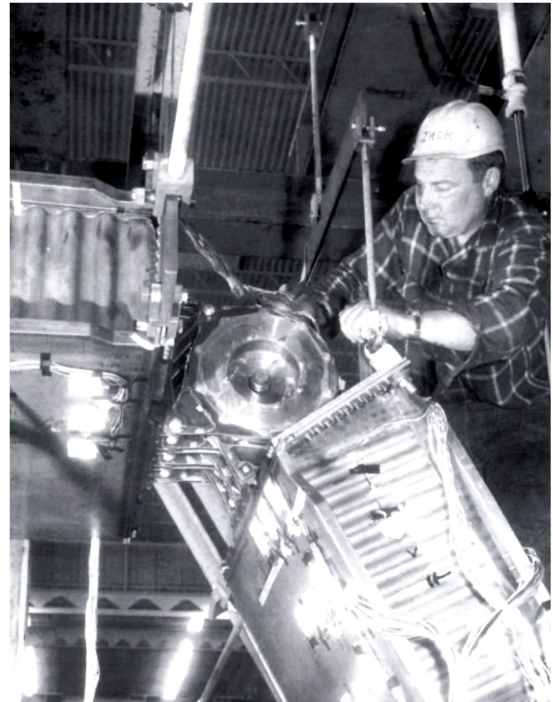
(c) XB-70 power hinge fitted within the wing box with an operator for size comparison
