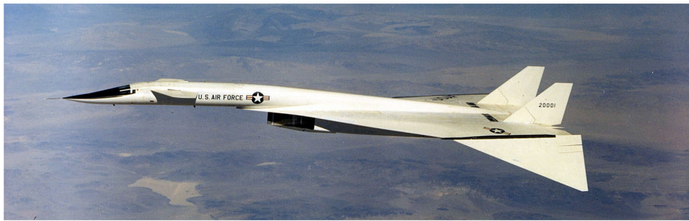
Fig. 2 The XB-70 AV-1 in flight, with wingtips folded 25° downward at low supersonic speeds.
