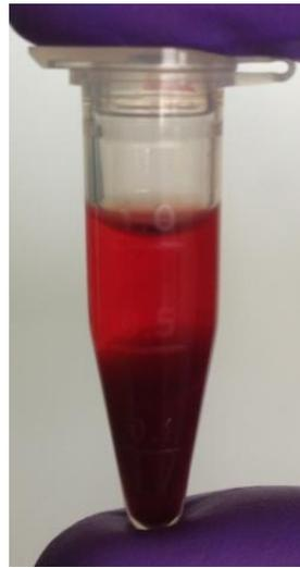
**Figure 3.19: Transparent red plasma after defibrinated whole horse blood was centrifuged at 5,000 RPM for 15 minutes.**
