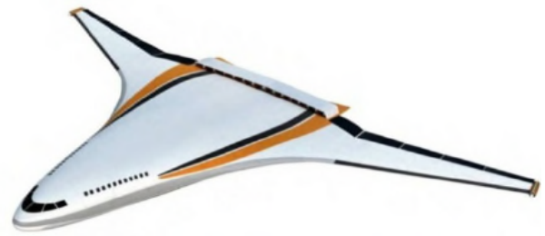
Figure 6 TeDP on a blended wing body airframe [47]
