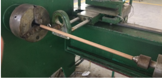
Figure 5: Mandrel mounted on machine
