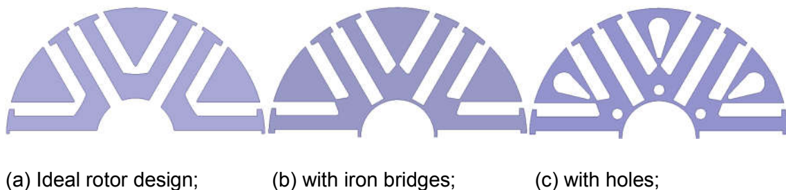
Figure 6-1 Rotor models with and without iron bridges.
