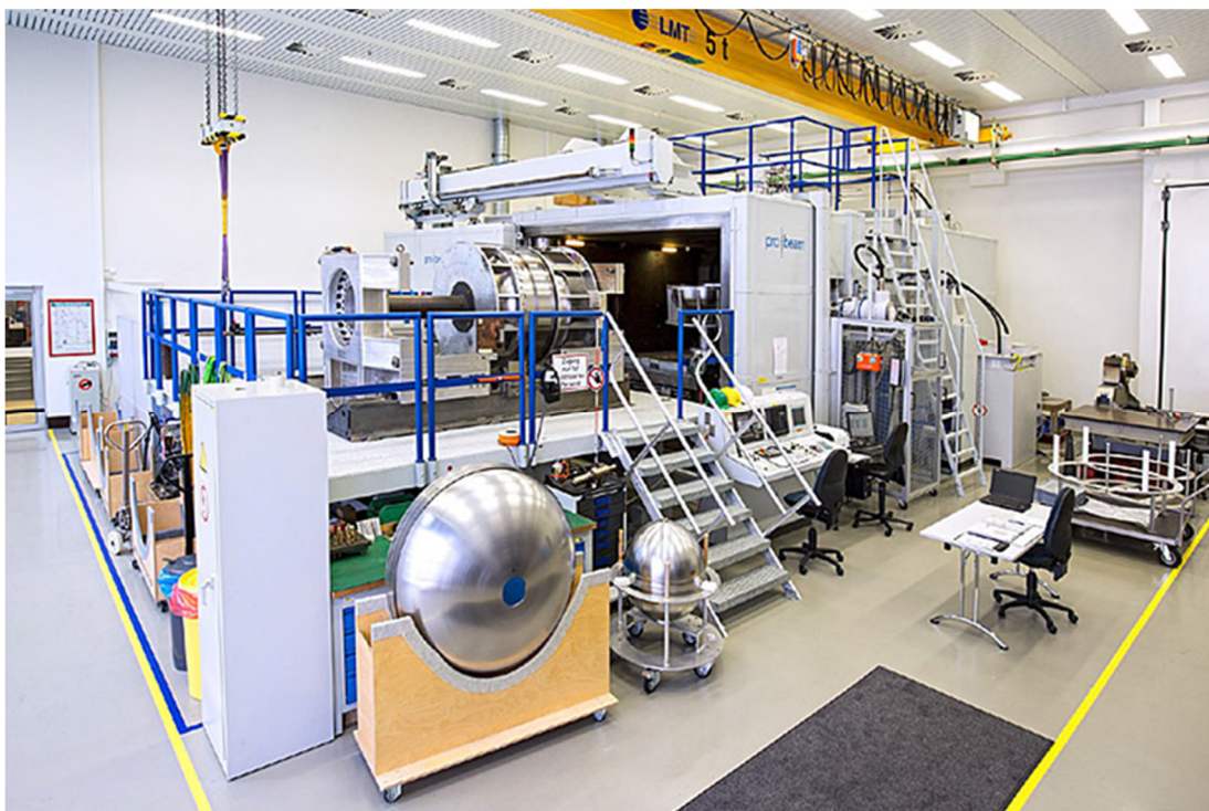
Figure 3 – Steigerwald Electron Beam Welding facility at EADS Astrium GmbH (Bremen) [6] .
