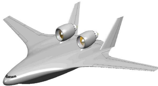
FIGURE 4.1: The NASA N2A BWB aircraft with podded nacelles 96
