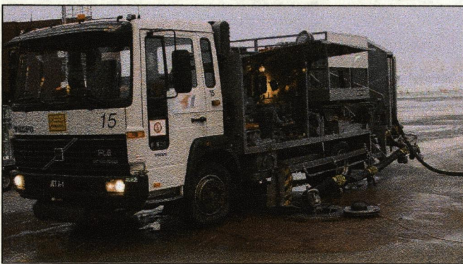
Figure 5-17. Dispenser truck in operation during refuelling. (Photo by Michael Bracha, 2002, Linde Gas, Germany)
