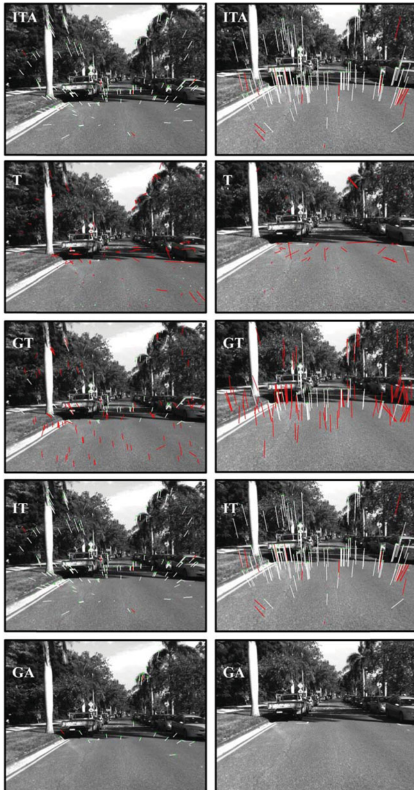
Fig. 10. 2nd Humped crossing case: white optical flow-inliers; red optical flow-outliers; green current position of the tracked feature.
