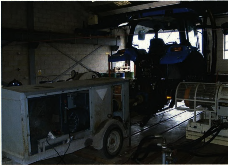
Figure 9-3 – Test tractor undertaking dynamic power boost investigation with axle and P.T.O. dynamometers
