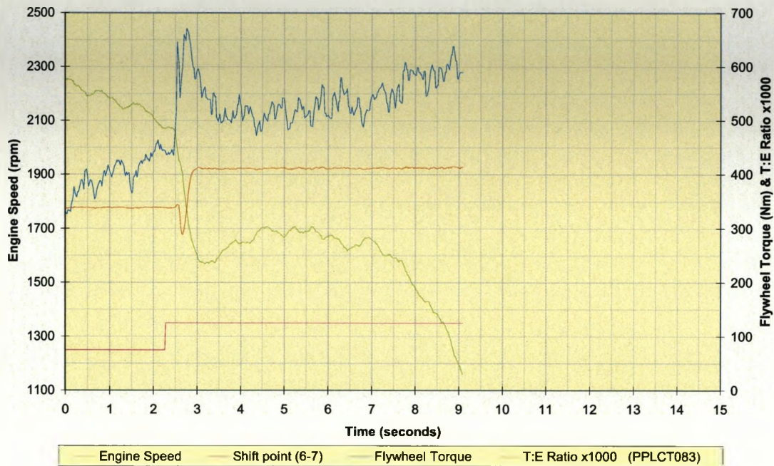
Figure 5-14 – The effect of a 6-7 gearshift whilst ploughing clay soil (406mm furrow width)
