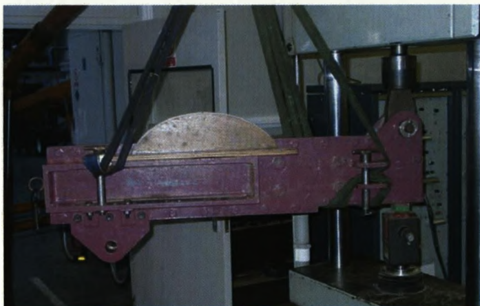
Figure A3.3– Left leg of Scholtz linkage ready for calibration of H_L
