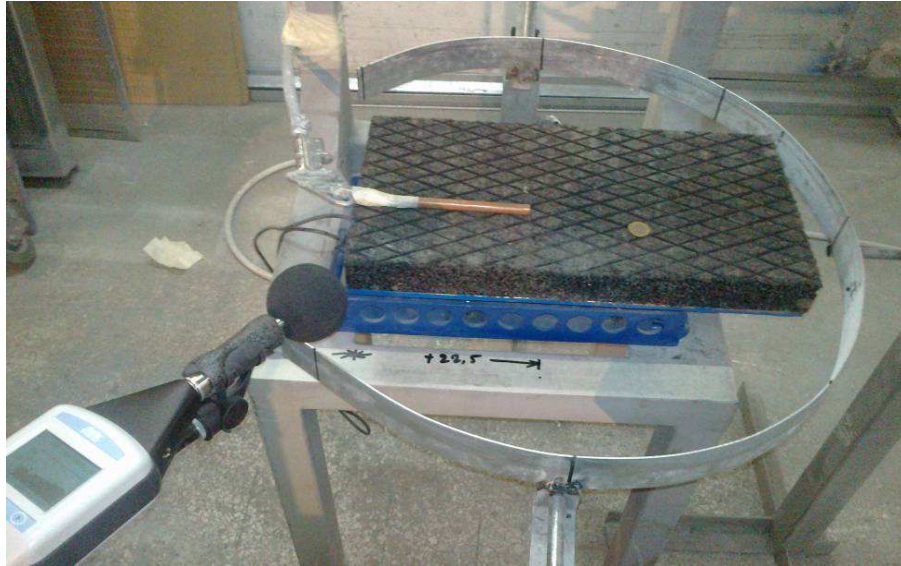
Fig. 10-41 Measurement - Only pipe over porous surface
