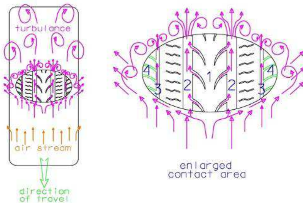
Fig. 2-25. Schematic of air turbulence
