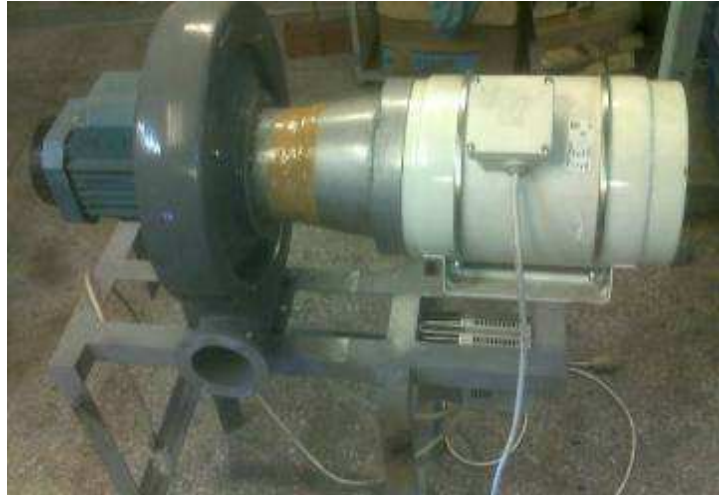
Fig. 5-19. Auxillary fan mounted on main high pressure fan
