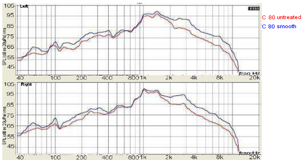
Fig. 7-8. Tyre C over smooth and over untreated surface at 80km/h
