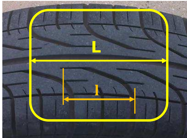
Fig. 7-22. Estimated tyre/pavement contact area
