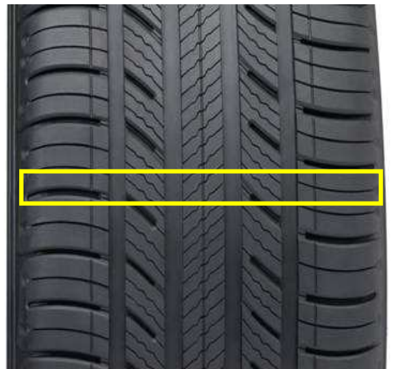
Fig. 3-6 Rubber blocks – Actual design (progressive)
