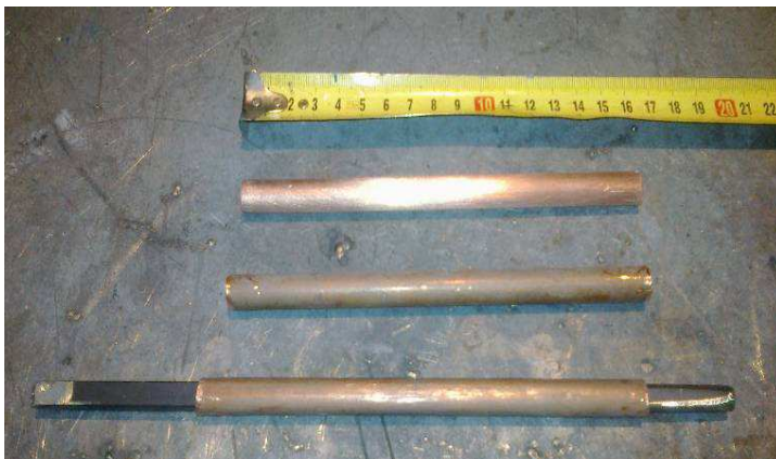
Fig. 10-9 Copper pipe - to simulate tyre groove
