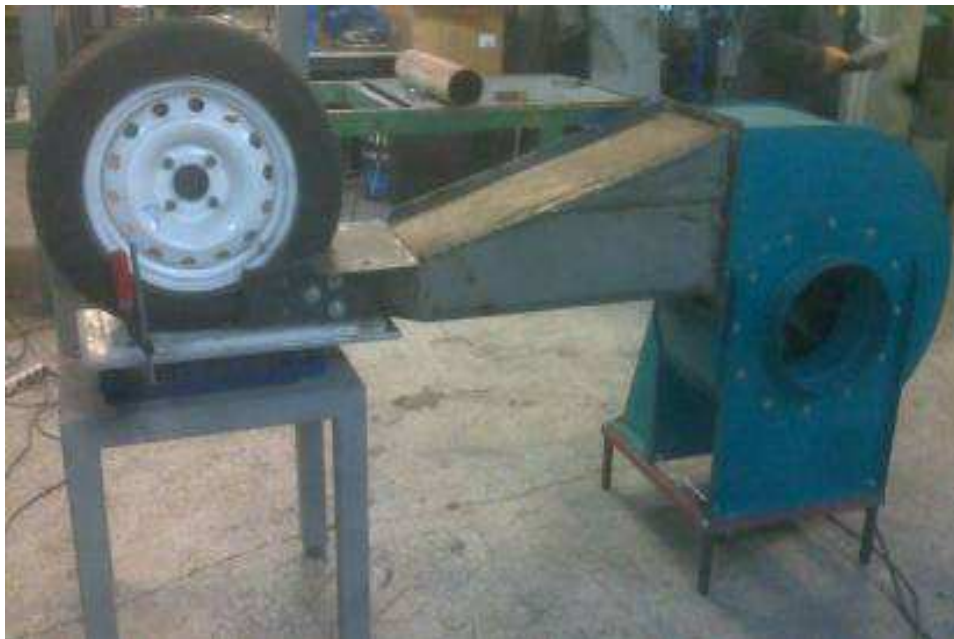
Fig. 5-18. Tyre mounted on rim & new high supply /low pressure fan
