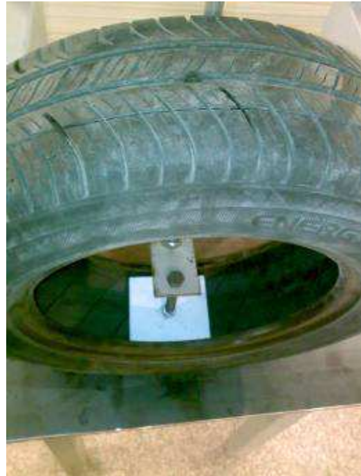
Fig. 5-8. Pressure pad inside tyre
