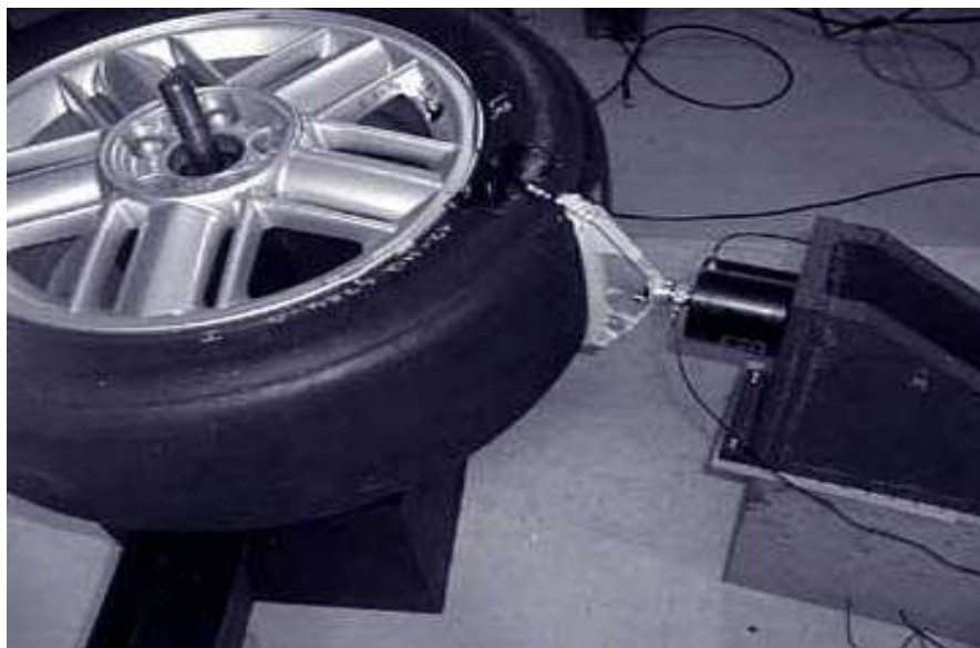
Fig. 2-6 Vibration setup from RATIN project of ISVR Research Center
