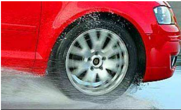
Fig. 3-15 Water mist at trailing edge
