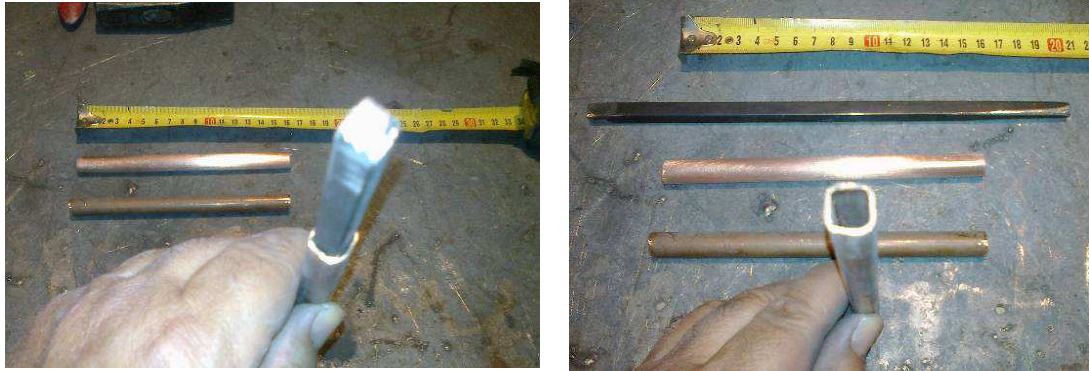
Fig. 10-8 Cross section from circle to rectangular
