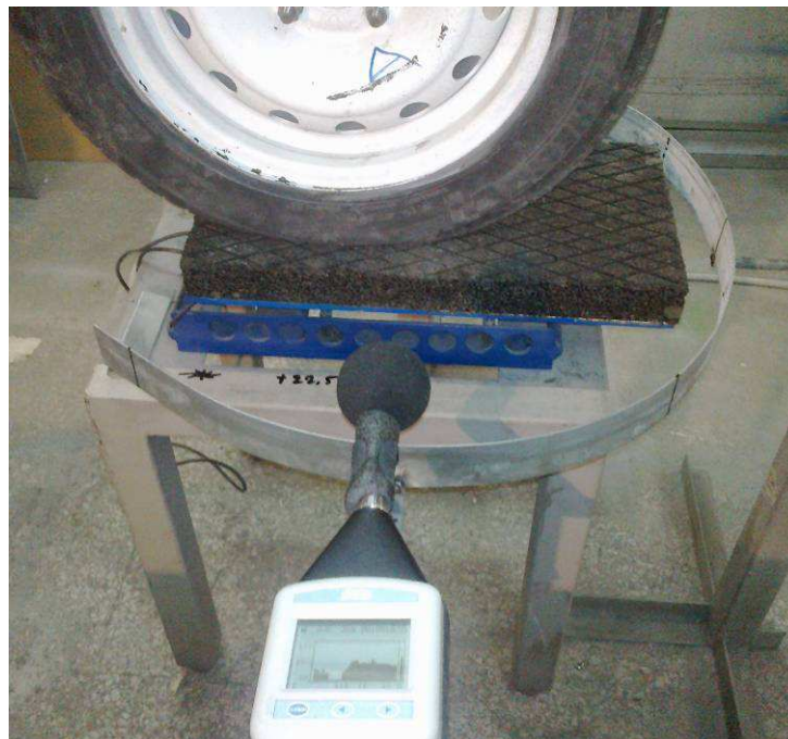
Fig. 10-42 Measurement - Pipe & tyre over porous surface
