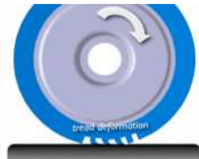
Fig. 3-5 Rubber blocks – Wrong design
