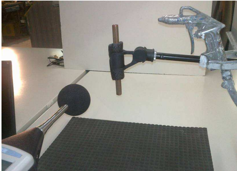
Fig. 10-10 Air stream at 90deg. to pipe
