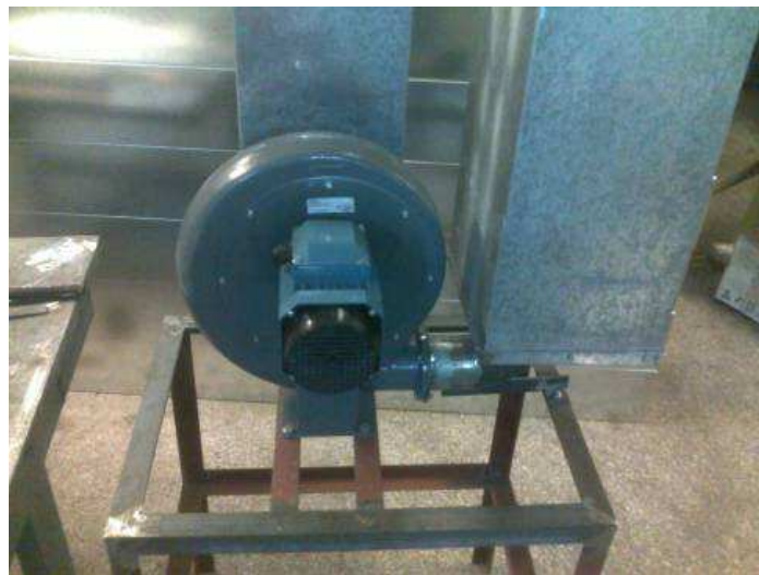
Fig. 5-15. High pressure fan regulated by a single face inverter (from 0-max rpm).
