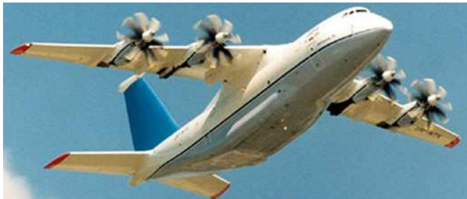
Figure 14: Wing mounted puller OR engine (Antonov An-70) [Ref. 122]
