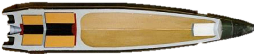
Figure 4-1 155mm M549A1 projectile with SRM [9]
