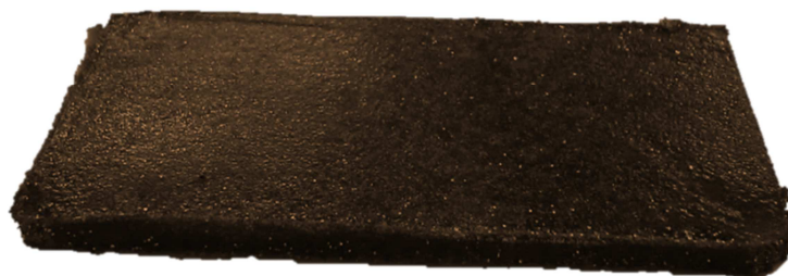
Figure 4-38: SRM propellant sheet for DMA specimens
