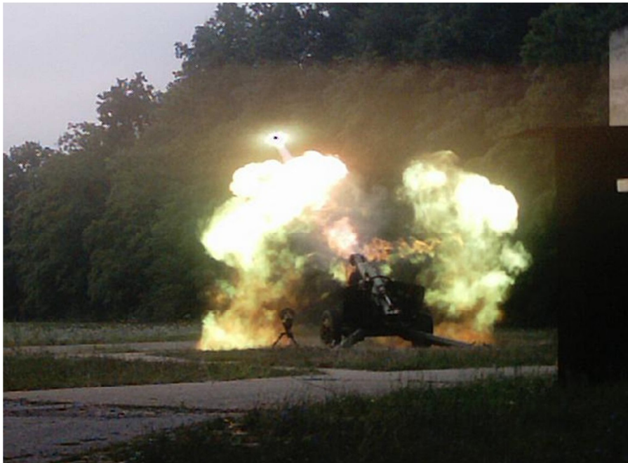
Figure 3-3 Testing of HE-ER/BB 105mm [38], observe burning of the BB just after the muzzle exit (no interim in burning)
