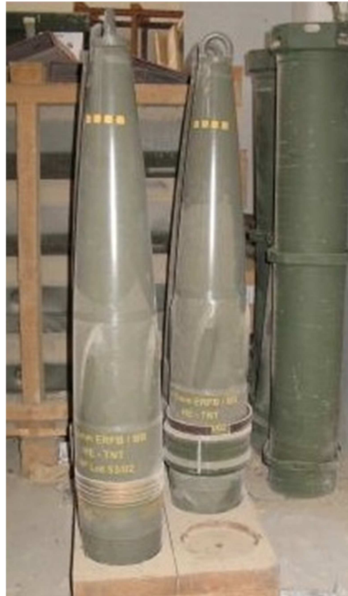
Figure 3-30 Projectile 155mm ERFB with base bleed unit [38]
