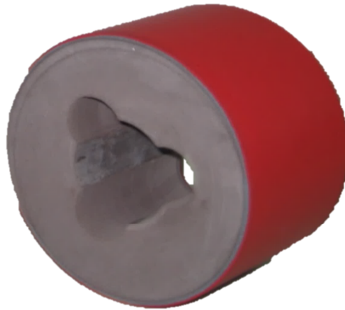
Figure 3-28 155mm experimental base bleed propellant grain [38]
