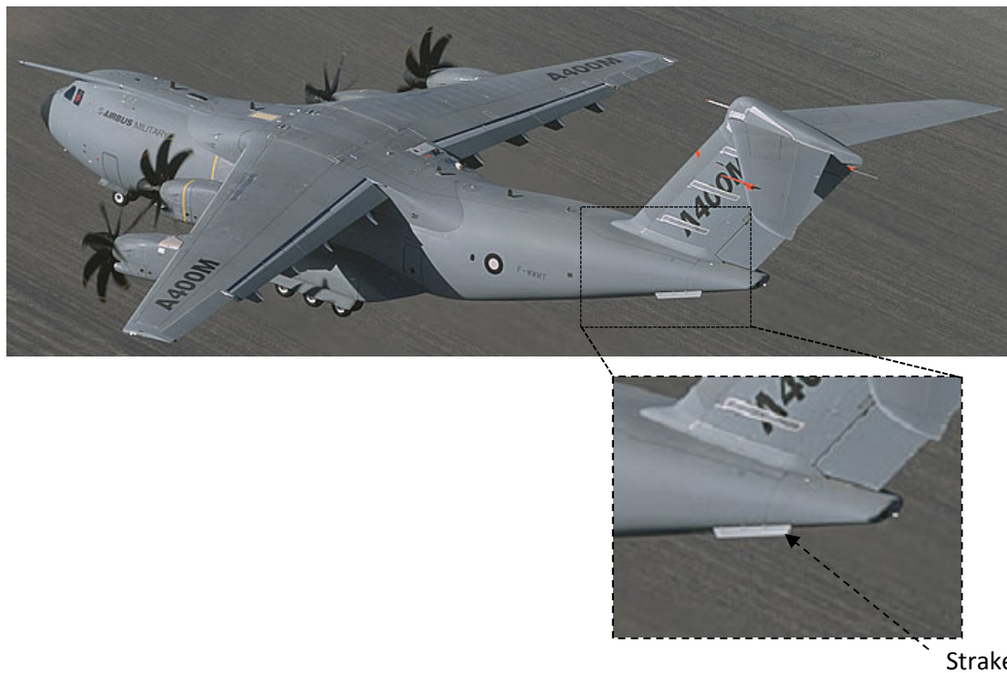
Figure 4-73 a) Separation area on rear fuselage of 10° configuration, b) strake on A400M rear fuselage potentially used to avoid separation [68]
