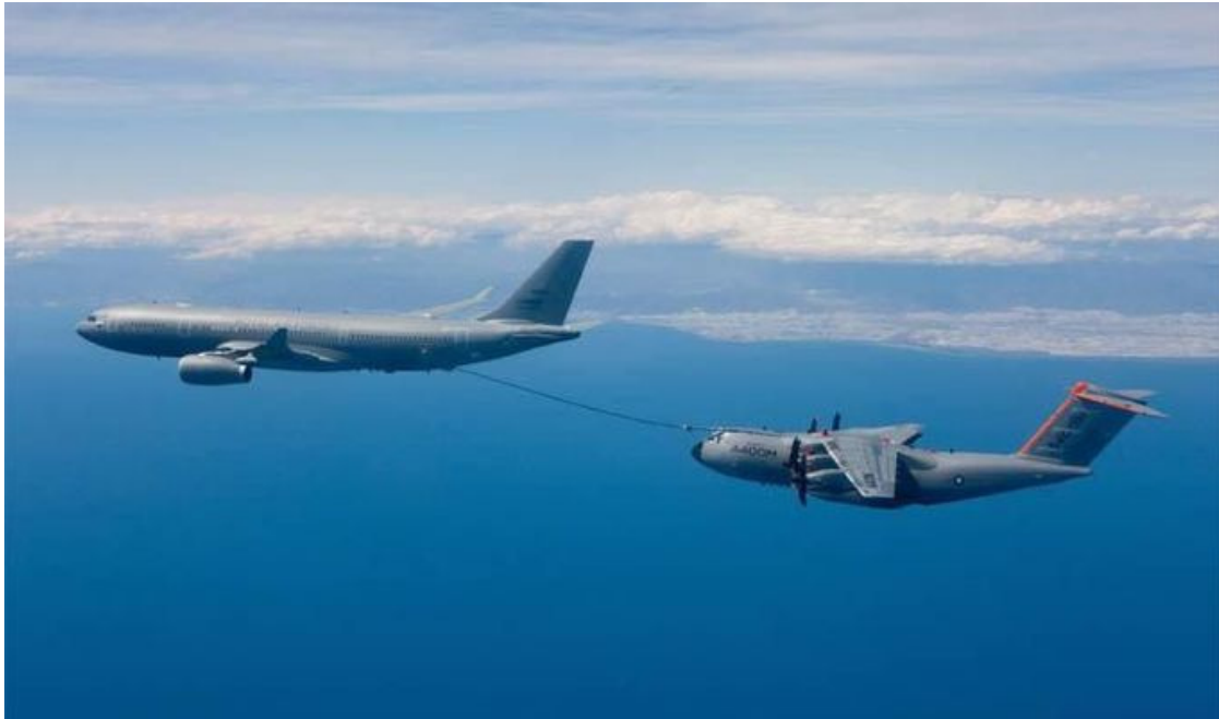
Figure 1-2 An A330 [54] refuelling tanker with an A400M [54] receiver aircraft during in-flight refuelling with a drogue and probe system [64]
