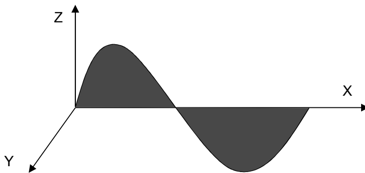
Figure 2-19 Sketch of a 2D wave with propagation direction in X, amplitudes in Z and no amplitudes in Y
