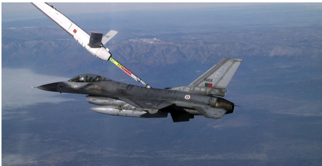
Figure 1-4 a) Flying boom system schematic refuelling configuration [57] b) Photograph of an F16 during in-flight refuelling with a flying boom system [58]
