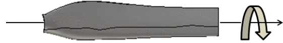
Figure 5: Blade position for a 0 degrees aspect angle. The blade is then rotated along its longer axis (indicated by the thin black arrow) and the RCS is calculated with CST with a step of 1 degree over 360 degrees. The image shows the CAD model of the blade that was imported into CST to carry out the simulations.
