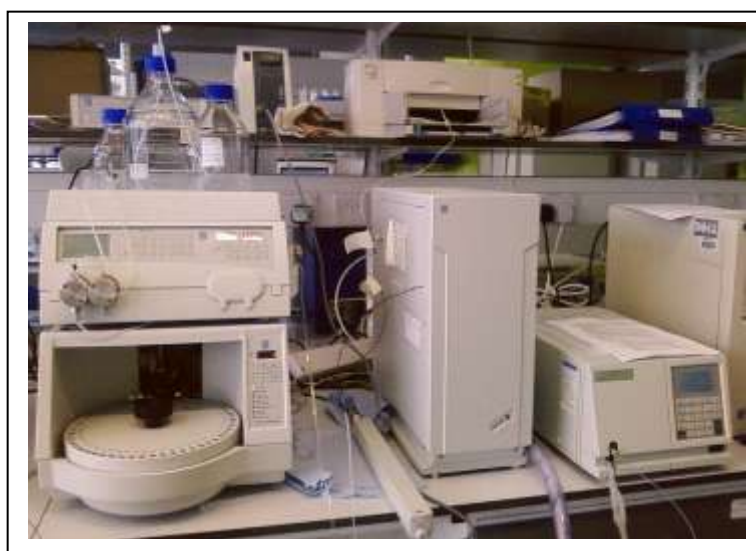
Figure 3.4. Dionex HPLC system.
