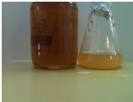
Figure 2.12 The colour change induced by bacterial growth in sterile growth medium.
