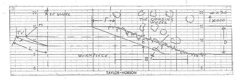
The grinding conditions are constant. The grinding wheel specification is Carborundum 5A-60-I8-V50.
