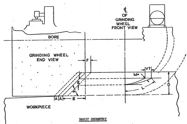
B = LOSS ON THE LEADING EDGE TO STABILISE ALPHA (~) THE APPROACH ANGLE
