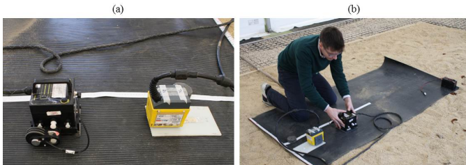
Fig. 1. Data acquisition detail. (a) GPR platforms. Left: 2GHz antenna; Right: 3GHz one. (b) Data collection over the surface pad.
