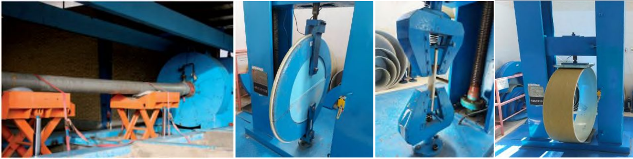
Fig. 4: Measuring Failure pressure, HTS, LTS and pipe stiffness (left to right)
