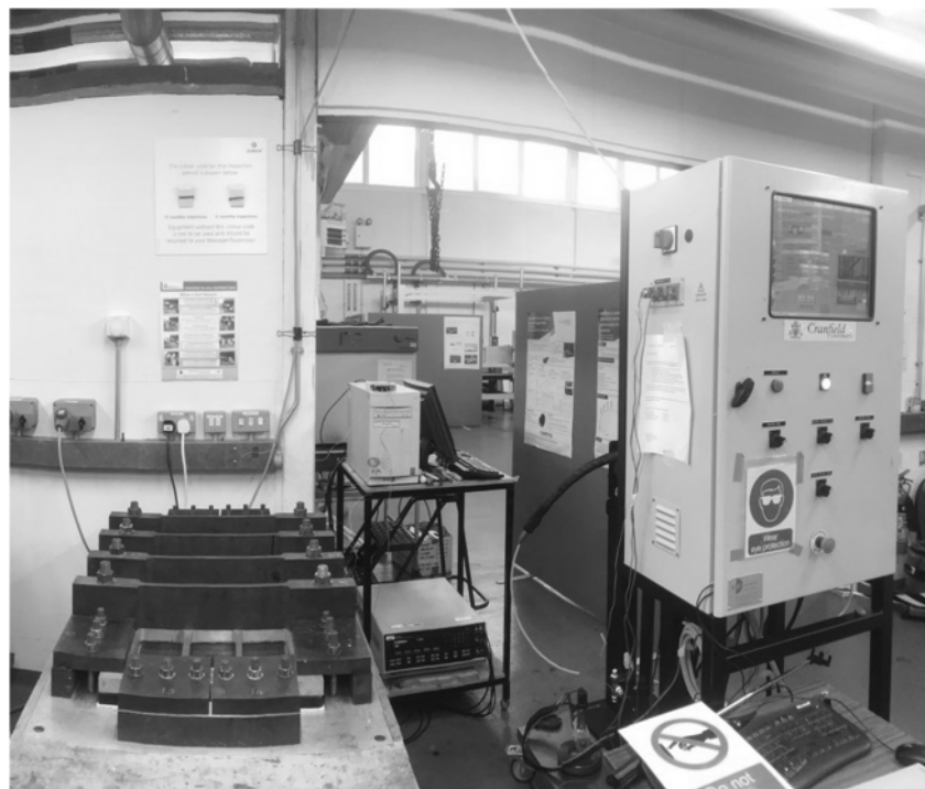
Figure 6 RTM tool, injection machine and data acquisition system.
