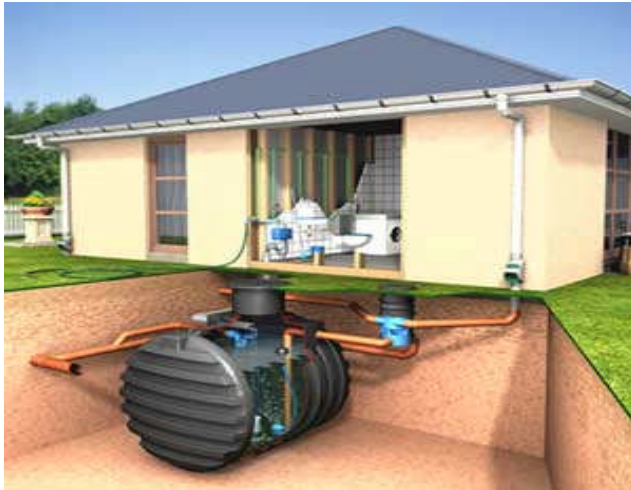
Figure 1. Illustration of rain water harvesting system
