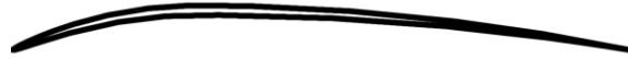
Figure 5-2 Inappropriately phrased optimisations can converge to give very thin and highly cambered solutions
