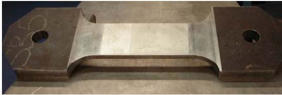
Fig. 1: BS EN 10025 Grade S275JR test specimen
