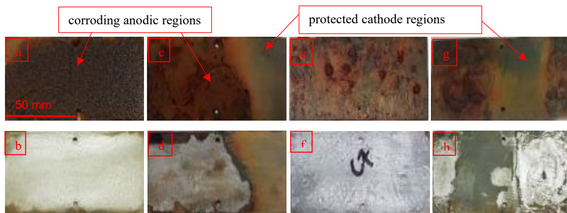
Figure 10 Pictorial view of the corroded and chemically cleaned steel coupons (C-series) collected from artificial seawater. Here exposure periods are as follows: (a, b) 45 days (c, d) 90 days (e, f) 210 days and (g, h) 321 days
