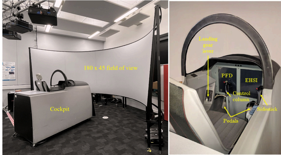
Fig. 2 Overall setup (left) and cockpit environment (right) of the EFS500 flight simulator.
