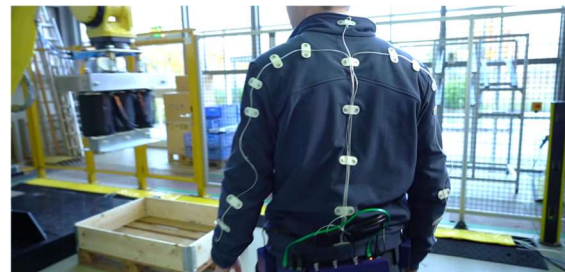
Fig. 5 Prototype of the motion capturing system used for human shape reconstruction (Source: BIBA)
