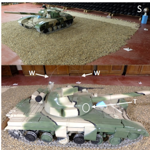
FIGURE 5 | Photographs of model tank target. The wire on top is denoted by “W”, the turret of tank denoted by “T” and the reference sphere is denoted by “S”.
