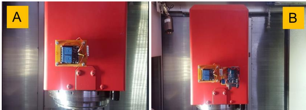
Figure 26: Prototype implementation of modular IoT DAQ unit
