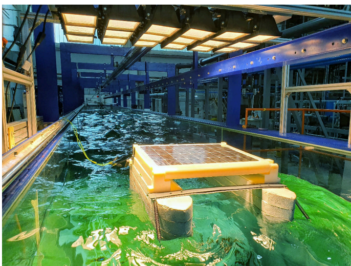
FIGURE 3: Combined solar simulator and wave tank facility at Cranfield University
