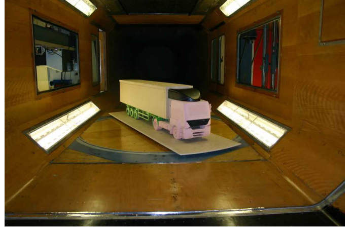
Fig. 3. Cranfield 8' x 6' model installation arrangement.
