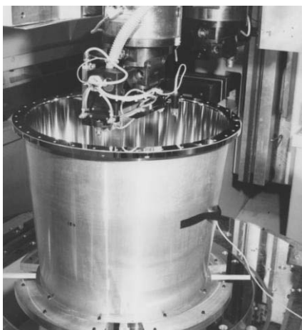
Fig.6: Rosat EUV mirror being measured on CUPE LDTM prior to NC error correct diamond turning
