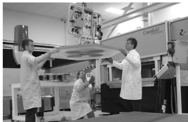
Fig. 9: Rapid production of large scale mirror segment using the – BoX® Cranfield ultra precision grinding/measuring machine
