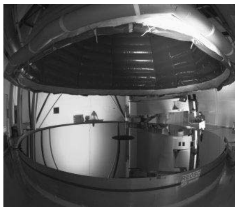
Fig. 2: VLT Mirror (8 m) undergoing optical measurement using in-situ measuring tower [9]
