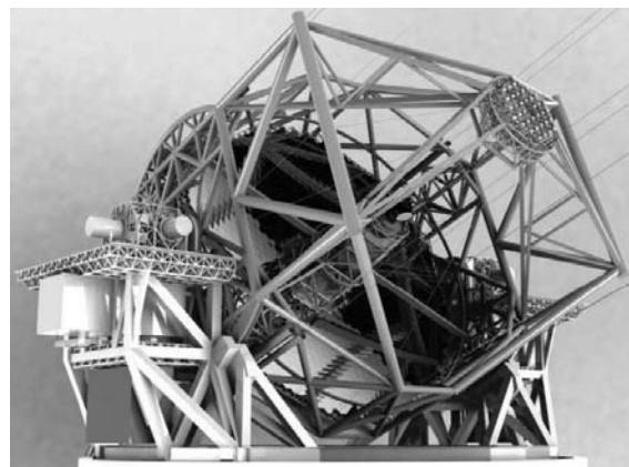
Fig. 1: European Extremely Large Telescope (42 m segmented primary mirror)
