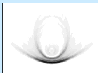
Kinetic Energy Distribution for a Shell Travelling at 300 m/s
