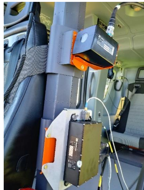
Figure 5: RT-TipTrak (top) and HT-VMU (bottom) mounted to the central pillar on the H135.
