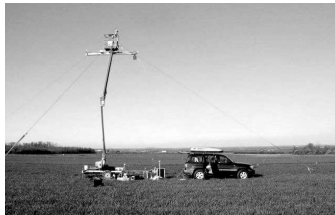
Fig. 7. Photograph of GB-SAR outdoor facility, with the linear scanner mounted on a 10-m-high hoist.
