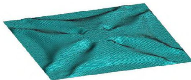
(b) Shape optimisation of a sheet subject to out-of-plane loads (reprinting permission for these images has been obtained from the publisher [158]).
