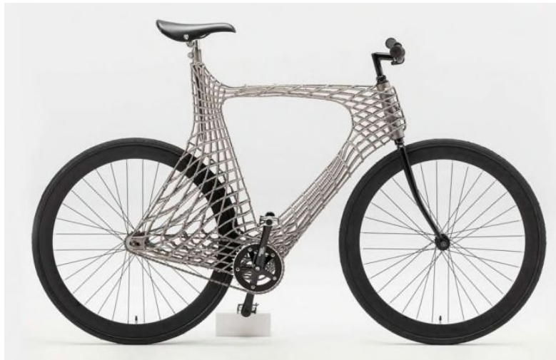
Figure 10: An example of a gridshell structure (a bike frame) made by a ‘dot-to-dot’ mode of welding using WAAM (reprinting permission for this image has been obtained from the publisher [156]).
