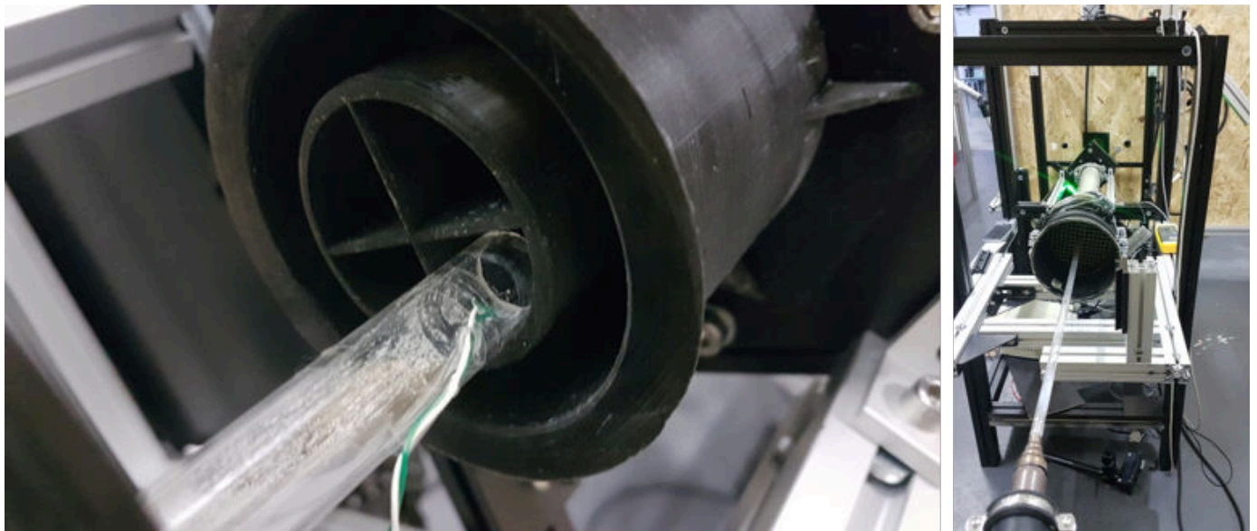
Figure 9. Glas tube inserted in one of the channels of the swirl generator for insertion of a hot flow streak. The cables sleeves visible are for a temperature sensor mounted at the tip of the glas tube(left). Inlet configuration for hot streak measurments with glas tube inserted in one of the channels of the swirler (right).
