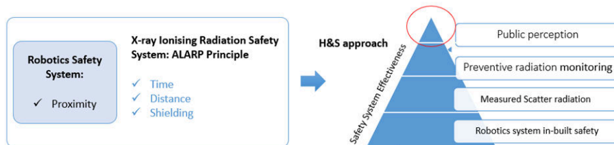
Figure 3: H&S clearance approach for robotic open cell concept with low power X-Ray
