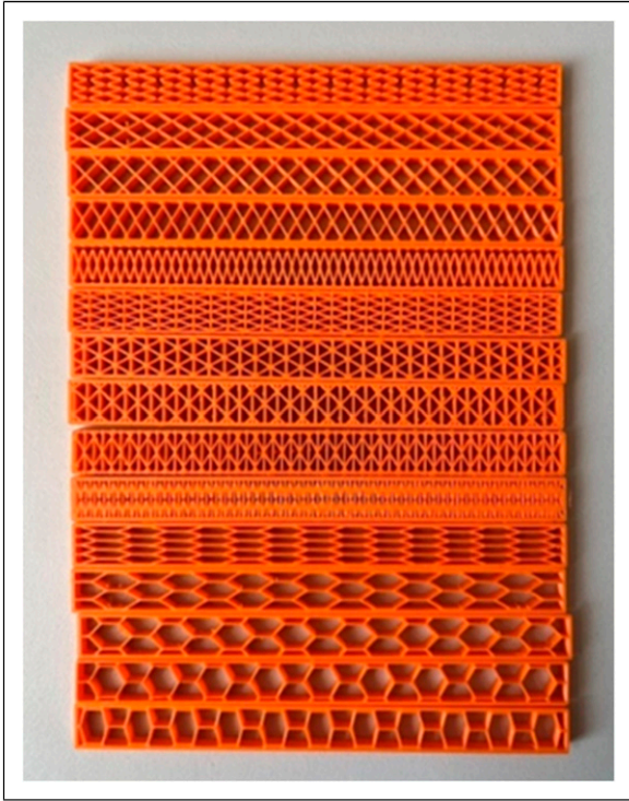
Figure 3. Schematic of the printed specimens with the different infill patterns and infill line angles.
