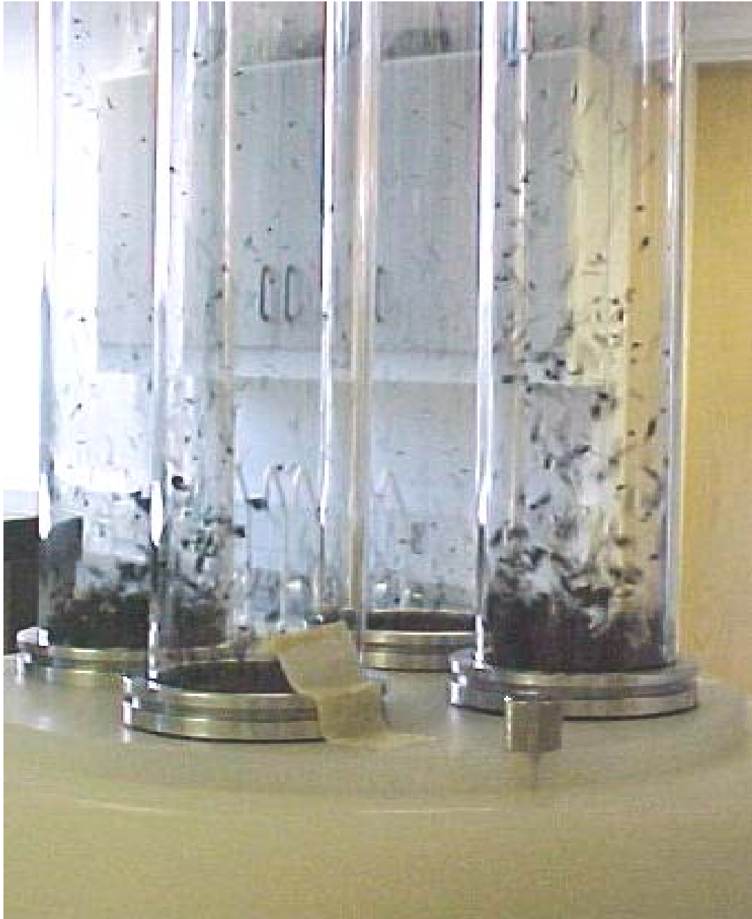
Plate 2.1. Fluidised bed dryer 350s (Burkard Manufacturing Co. Ltd, Hertfordshire, UK) that was used in the studies
